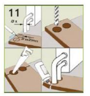
If, for example, heating pipes protrude from the floor, first cut the board to the right length. Then lay the board piece next to the actual location and measure and mark the recesses with the bending rule. Again, don't forget to leave a gap of at least 10 mm around the expansion joint. You can now drill the marked areas. Then saw the board at a 45° angle. This method enlarges the place to be glued. Then place it behind the heating pipe and join it back to the board.
