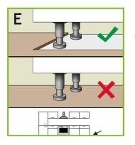
Fitted kitchens and built-in cabinets must be assembled prior to installation. Installation over flooring is not permitted.
