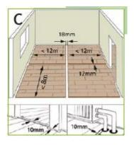
In rooms that are more than 12 m long in length and/or more than 8 m wide in breadth, an expansion joint must be used. This also applies to doors, room openings, wall projections and passageways.
