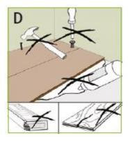
The floor is installed as a floating floor. Boards must not be glued, nailed or otherwise attached to the subfloor. As wood is a natural material, the flooring will work perfectly. Thanks to the floating installation and the distance between the walls, give the installed surface the possibility of minimal movement.
