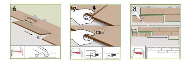
The joint offset between rows should also be at least 40 cm to ensure that the tongue connection and groove connection keep stable. Simply place the panel at an acute angle to the installed panel and push it in until it audibly clicks into place. The angle is correct when the panels can be assembled easily without any force.
