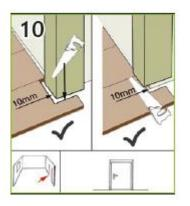
Wooden door frames can be shortened. To do this, place a board against the frame with the decorative side down. Now shorten the door frame with an appropriate saw along the board. Then the board can simply be pushed under the frame with the decorative side up. For door frames that cannot be shortened, cut the panel to size accordingly.
