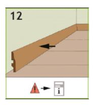
Skirting boards will be fastened to the wall, not to the floor.
