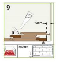
The last row usually needs to be adjusted in length. Meanwhile pay attention to the distance to the wall and cut the panels appropriately. If the panel is too wide, it should be adjusted lengthwise.
