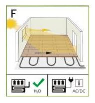
Out of optical reasons, the laminate should always be installed lengthwise to the main light source. Before laying, calculate the width of the last row of panels. It should not be narrower than 5 cm. Cut the first row to the appropriate length.
