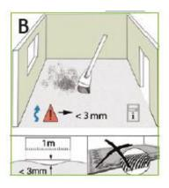
The substrate must be free of cracks, clean, tension/pressure resistant and permanently dry (VOB, Teil C, DIN 18365). Old coatings must be completely removed from the substrate, as they affect the flatness of the substrate. The flatness of the substrate must not vary by more than +/-3 mm over 1 m (DIN 18202). If possible let the underlayment be checked through the floor layers
