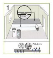
For screeds and concrete floors, first install a vapor barrier parallel to the laminate. You can either let the film strips overlap by 20 cm or glue them end to end. In any case, it should overlap the walls by approximately 3 cm.
